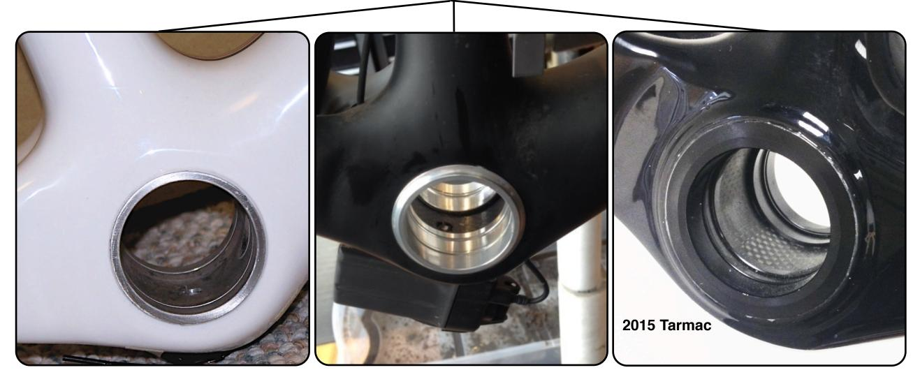
These are the 3 versions of OSBB Road that utilized an Aluminum Inner Shell over the years. This is essentially a 68mm BB30 frame that is 68mm Wide X 42mm Diameter.
